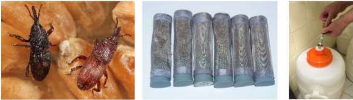
Figure 49 Grain weevils in different developmental stages were placed in cages inside hermetic containers to investigate the oxygen consumption to improve hermetic grain storage. (Photos: V. Misgaiski and C. Müller-Blenkle, JKI)
